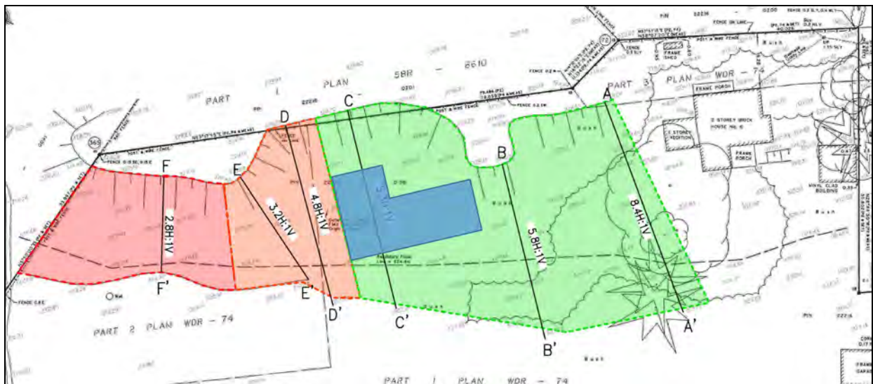
Figure 4: House location (in blue) on topographical base with slope conditions indicated (source: MHBC, with input from Chung & Vander Doelen)
